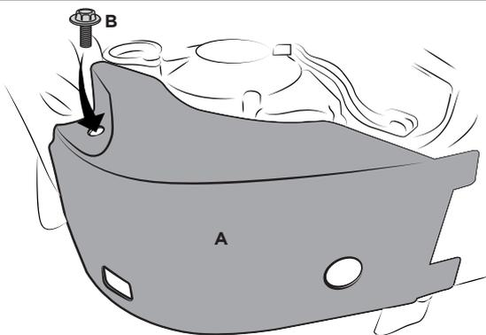
**Fix the skid plate (A) with the screw (B).**
